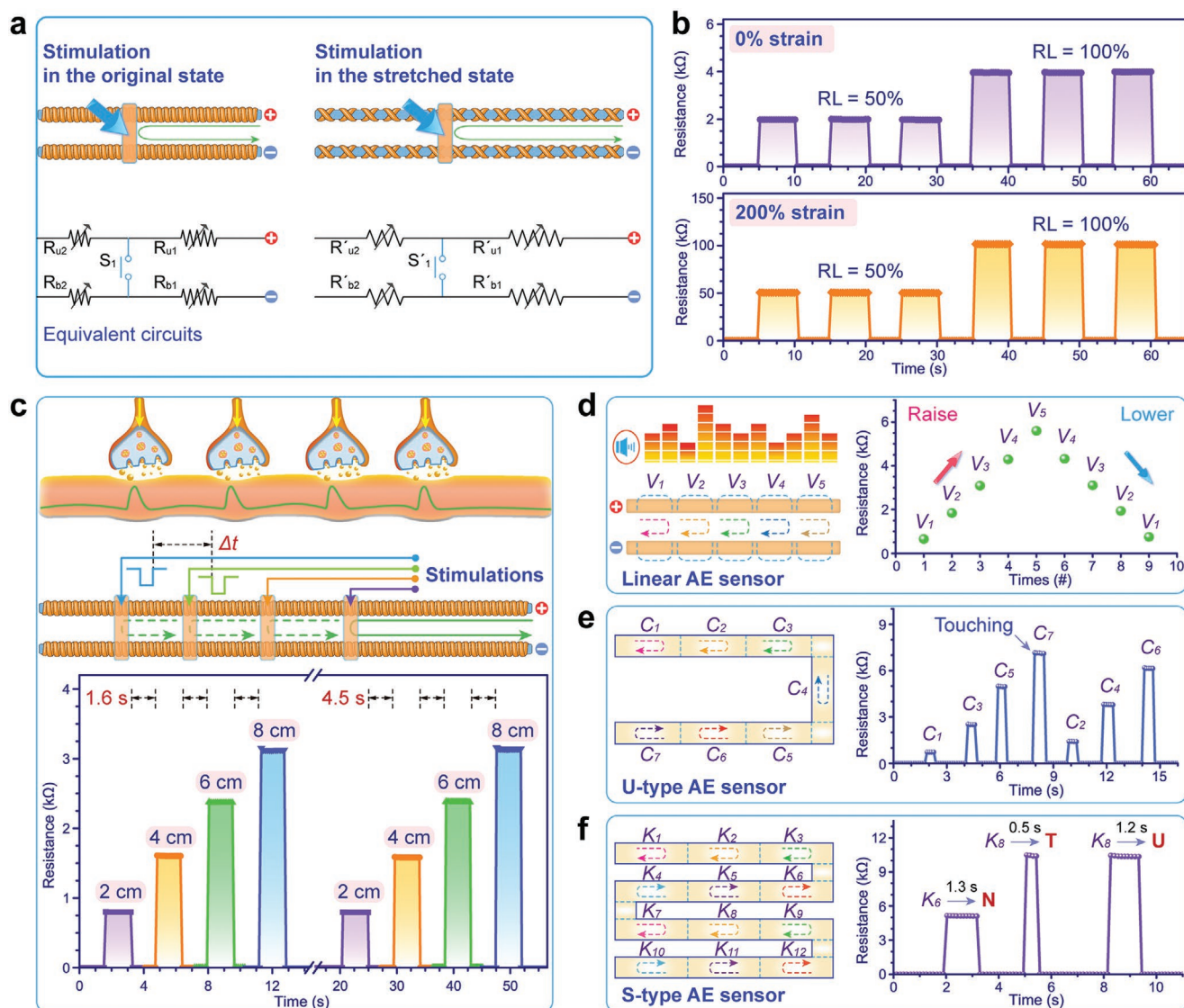
Figure 3. Performance and characteristics of the AE sensor. a) The working mechanism of the AE sensor in the original state and stretched state and their corresponding equivalent circuits. Longer effective working length by stretching the AE sensor brought more available portion to perceive the external mechanical stimulation. b) The change in the response resistance versus RL, where the external mechanical stimulation is applied on the original and stretched AE sensor, respectively. c) Spatiotemporally dynamic stimulations applying on the AE sensor. Top: Diagram of biological synapses and the AE sensor subjected to the external mechanical stimulation. Bottom: Repetitive responses to the dynamic stimulation applied on different location of the AE sensor at the interval time of 1.6 and 4.5 s, respectively. d) Music control demonstrated by using a linear AE sensor. e) A U-type AE sensor used for playing game and its typical resistance responses. f) Wireless typing based on an S-type AE sensor and its typical resistance responses.
